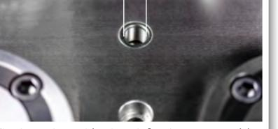
Thanks to the probing bore hole, the centre position of the zero clamping system can be determinded extremely quickly and easily.
