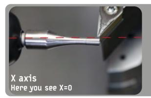
Without any further calculation, you measure your tools to the centre of the spindle, respectively X=0.
