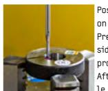
Position the tester approximately on the centre of the circle. Preselect if you want to probe inside or outside and give an approximate diameter.
