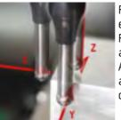
Position the tester in front of the edge. Preselect axis X, Y or Z, as well as the direction + or - . After starting, the cycle probes automatically and writes into the offset - that's it!
