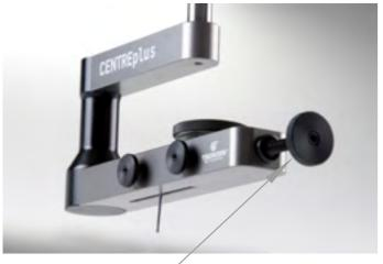
Fine adjustment: With the fine adjustment, you can position the dial gauge precisely.
