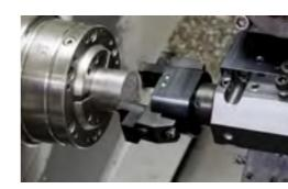
Position the bar gripper in Z axis in front of the bar.
