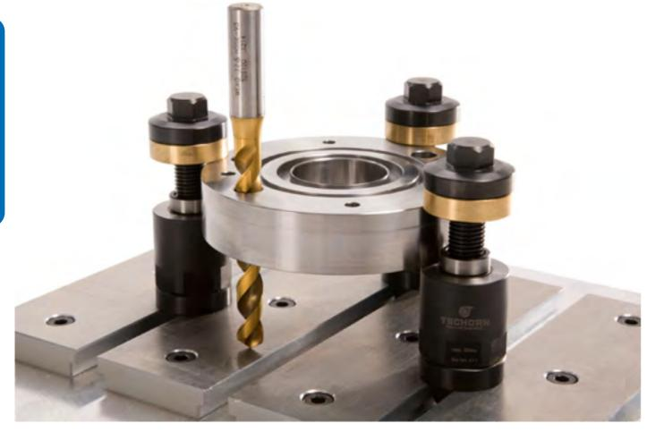
**Quick setting with the clamping bolts:** move each single bolt without clamping screw into the slide block of the machine table and position the bolt by hand as a stopper at the workpiece. Tighten the clamping bolt and it automatically helps you to position the workpiece.
