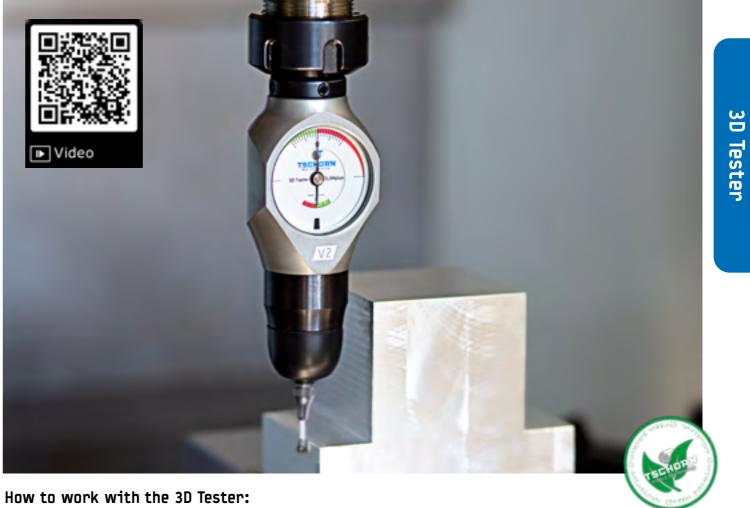
Clamp the 3D Tester into your tool holder. Adjust the run-out as explained in the manual. Approach your workpiece with the 3D Tester. As soon as the indicators show "O", the spindle axis precisely stands on the workpiece edge.
