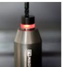
Chose the milling tool you want to measure and start the cycle. After starting, the cycle automatically probes the tool length and writes the tool length into the tool offset of the machine.
