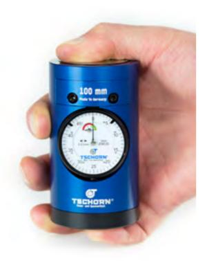
Simple adjustment: Push tester Small indicator at -2 mm Turn scale for large indicator to 0 Ready:
