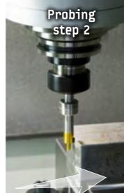
2. By slowly and carefully approaching the rotating edge finder to the respective reference surface, the oscillation movement steadies successively.
