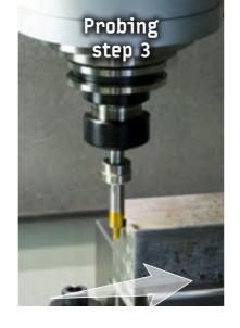
3. When reaching the final position, the edge finder body passes along the edge. Now, the position corresponds to the radius of the tracer.
