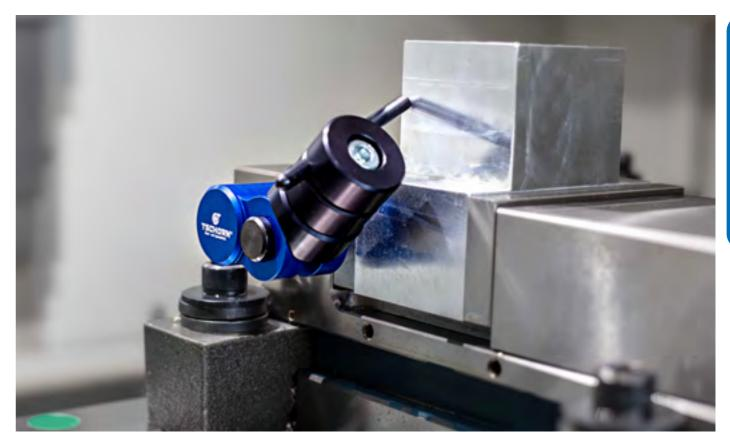
With its built-in magnets the workpiece stopper gets fixed directly to a bench vice (for example) and applies for exact positioning of your workpiece. After clamping, it can simply be removed and releases the positioning surface for processing.
