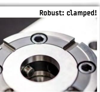
Up to 4 clamping screws can be used on each clamping pot to clamp the locating bolts - usually, one clamping screw per clamping pot is enough for a secure clamping.
