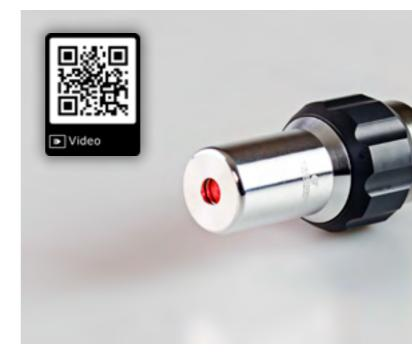
With the laserfinder, workpiece positions can be determined very quickly and easily without any direct contact to the workpiece. It is particularly suitable for determining rough workpieces e.g. for raw materials with allowance. Furthermore, the laser cross is also well suited to find the approximate centre of a round workpiece.
