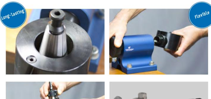
The assembly system is not only time-saving but also helps you to have longlasting tool holders: thanks to our unique technology, the tool holder is not clamped at its precise conus - the conus is free. This is safer for your tool holders and no damanges ensure a precise processing of the parts you have to manufacture.
